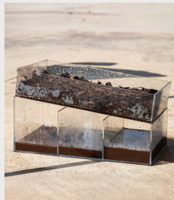
A SIDE-BY-SIDE DEMONSTRATION HELPS ILLUSTRATE THE DIFFERENCE IN WASH OFF BETWEEN WET MULCH AND MULCH GIVEN A FULL DAY TO DRY.
